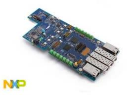
The NXP SJA1110 Ethernet switch has safety capabilities built in, offering integrated 100BASE-T1 PHYs, hardware-assisted security as well as multi-gigabit interfaces.
