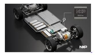
By leveraging NXP's advanced GD316x high-voltage (HV) isolated gate drivers, the solutions are designed to accelerate the adoption of 800-V and SiC power devices. Safe, efficient and higher performance traction inverters enabled by the GD316x product family can be designed to extend EV range and reduce the number of charging stops while lowering system level costs for OEMs.
