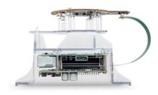
Designed to simplify the creation of new voice-control devices, the new NXP reference platform for Amazon Alexa on i.MX is a complete system containing Amazon's 7-microphone array design, far-field audio processing technology, and AVS client to enable customers and partners to create their own high performance devices with Alexa.
