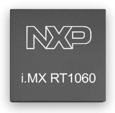
To address the need for smarter, more aware edge computing devices, the i.MX RT1060 processor delivers the highest performing Arm® Cortex®-M7 based devices with real-time operation and applications processor-level of functionality.
